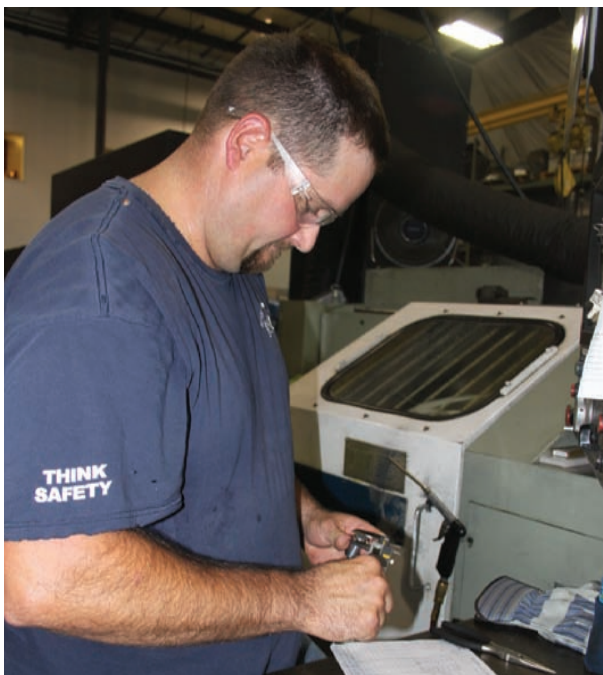
CNC Programmer Zac Way verifies a part's measurement with the print during an in-process inspection.
